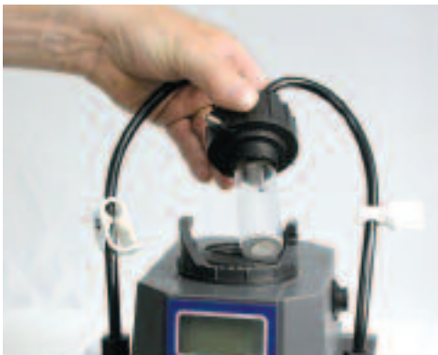
The flow-through sample cell is easily removed to insert a test standard.
